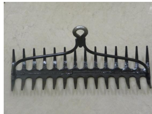
Figure 1. Picture of the double-headed rake used for point intercept aquatic plant surveys.
